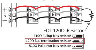
Use of appropriate shielded twisted pair wire (14-26 AWG) is recommended, per protocol specifications. Total wiring runs should not exceed 4000 feet, with a maximum of 128 devices (BACnet) or 32 devices (Modbus) in a single daisy chain.
